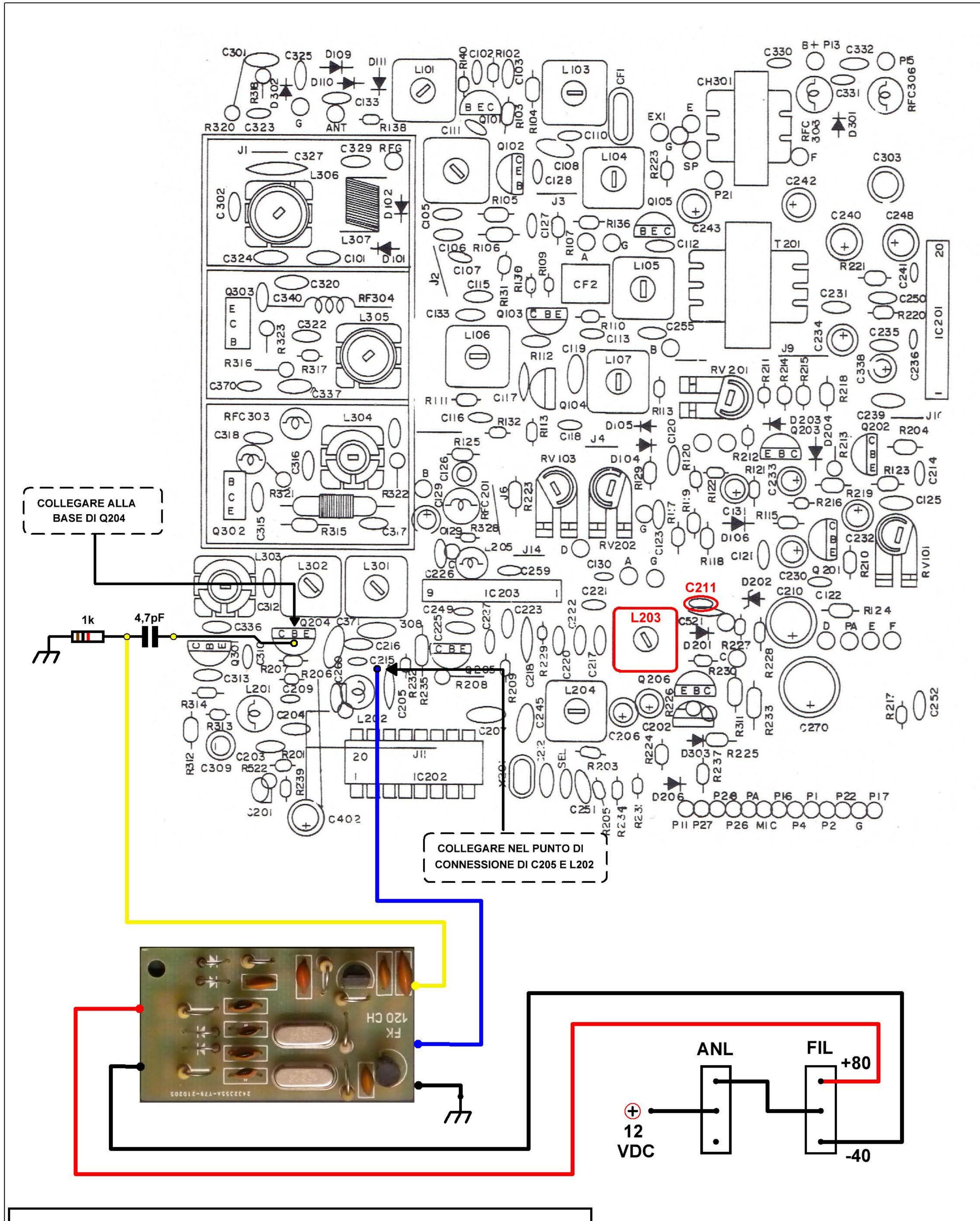
PER UN BUON AGGANCIO DI TUTTI I 120 CANALI E' PREFERIBILE SOSTITUIRE LA BOBINA L203 CON LA FALKON FK203 E SALDARE IN PARALLELO A C211 (LATO SALDATURE) UN CONDENSATORE CERAMICO DA 100pF.
